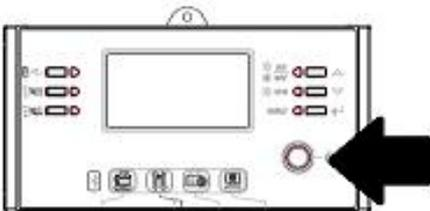
Step 4. Be sure to select battery type as "WEC" in LCD program 5.
