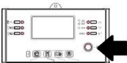
Step 5. Be sure to select battery type as "PYL" in LCD program 5.
