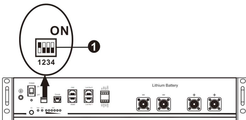
Dip Switch: There are 4 Dip Switches that sets different baud rate and battery group address. If switch position is turned to the "OFF" position, it means "0". If switch position is turned to the "ON" position, it means "1".
