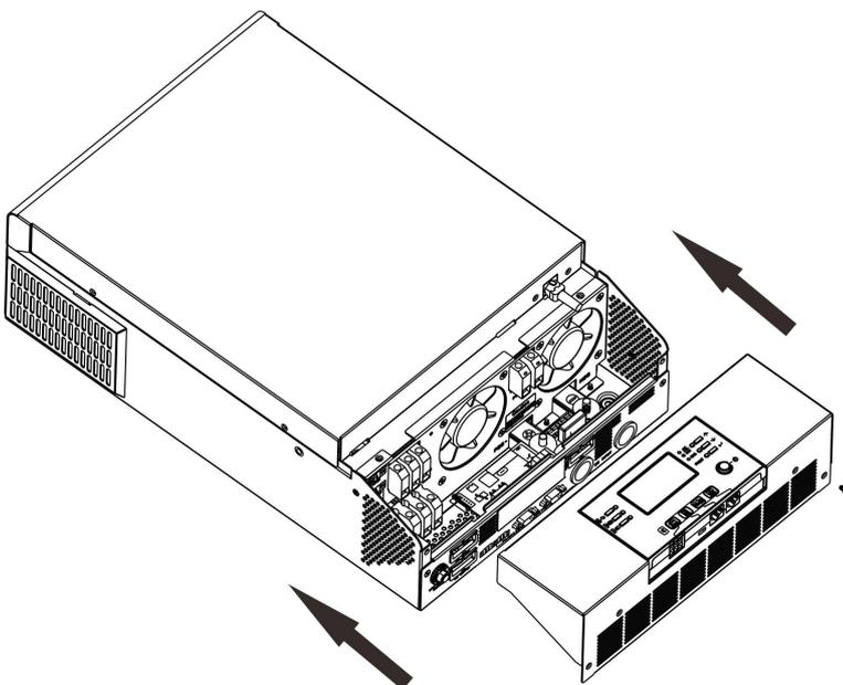
**Step 8:** Put wire cover back to the unit. Now the inverter is providing parallel operation function.
