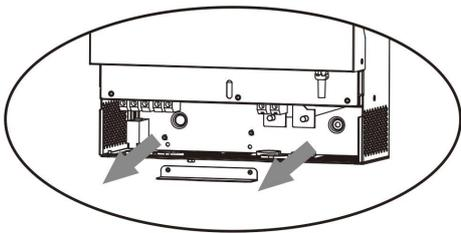
**Step 4:** Install new parallel board with 2 screws tightly.
