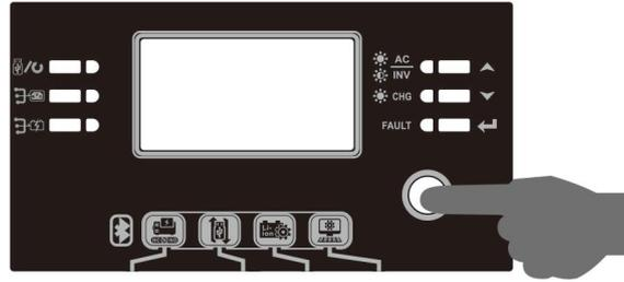
Once the unit has been properly installed and the batteries are connected well, simply press On/Off switch (located on the display panel) to turn on the unit.
