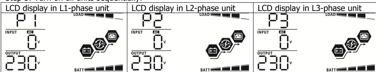
Step 4: Switch on all AC breakers of Line wires in AC input. If AC connection is detected and three phases are matched with unit setting, they will work normally. Otherwise, the AC icon will flash and they will not work in line mode.
