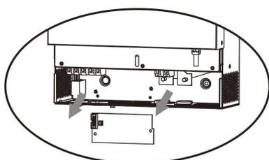
**Step 3:** Remove two screws as below chart to take out cover of parallel communication.
