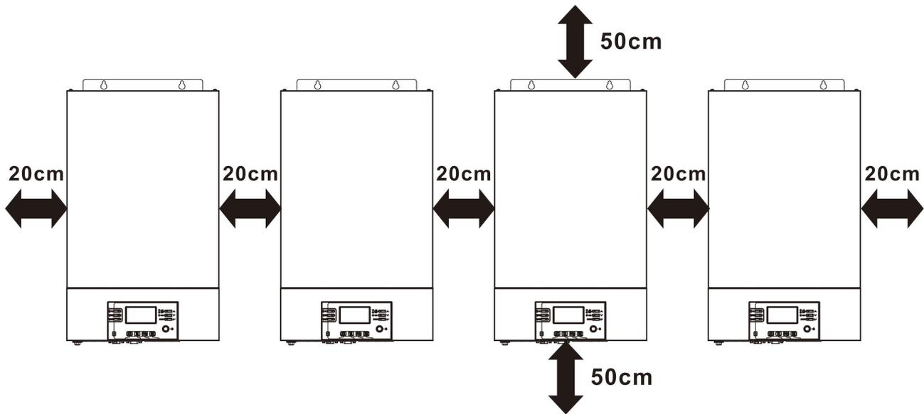
**NOTE:** For proper air circulation to dissipate heat, allow a clearance of approx. 20 cm to the side and approx. 50 cm above and below the unit. Be sure to install each unit in the same level.
