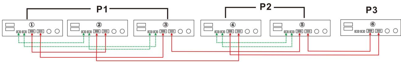
Three inverters in one phase and only one inverter for the remaining two phases:
